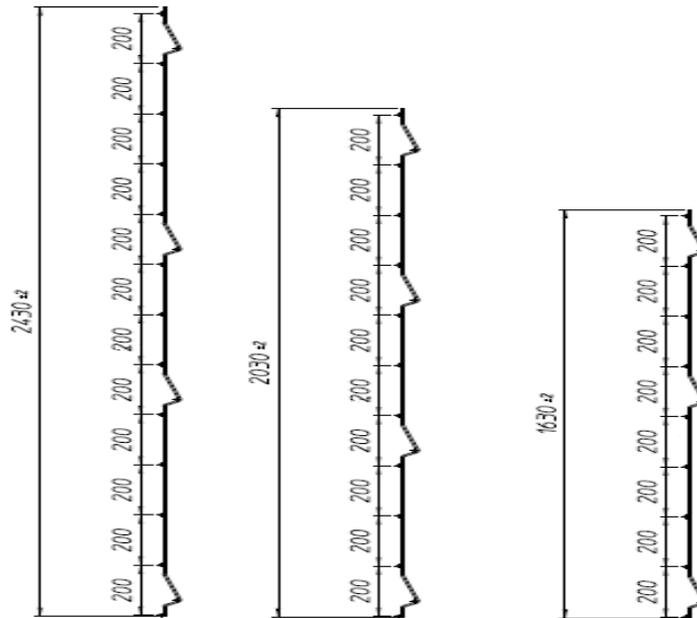
**Fig. 3: Dimensions of the panel**
